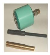
A selection of 89, 105 dia drum- and 125 dia biscuit Sicon Idlers manufactured from reprocessed UHMW-PE except the lower left 125 biscuit idler which was manufactured from virgin UHMW-PE material. Notice the 5 mm wear indicating hole in this idler.
