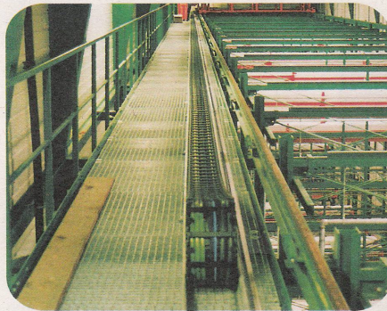
Storage and retrieval robot - the travel is 90 m, the speed is more than 4 m/s - igus® chains plus Chainflex® cables and guide troughs
