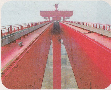
Gantry crane at shipyard - travel 185 m with igus® Rol E-Chain® Series 5050R E4/4 ► chapter 7 i More information on crane applications: igus-cranes.com
