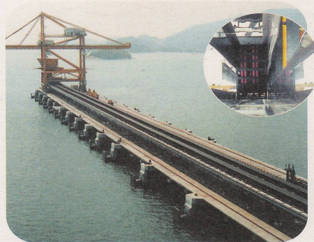
Cross-travel of 441.3 m, implemented with igus® Rol E-Chain® Series 5050R E4/4 ► chapter 7
